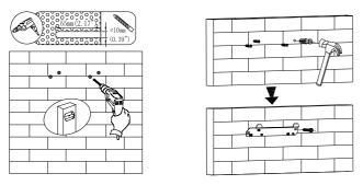
fig5.7 Wall mount installation diagram
