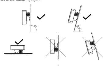
fig5.1 Installation diagram
