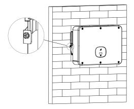
fig5.8 Inverter wall hanging diagram
