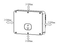
fig5.2 Mounting dimensions for an inverter
