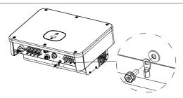
fig6.1 Grounding diagram
